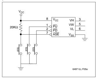
making a continuous push, after the first second, the increment/decrement speed increases. For the first second the device will be in the slow scan mode. Then if the button is held for longer than 1 second the device will be in the fast scan mode. As soon as the button is released the X9514 will return to a standby condition.
